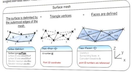
The surface type surfType is set to "TIN" when describing a triangular mesh. The presicion of the mesh model depends on the area2DSurf, 3D surface area area3DSurf and the elevation maximum elevMax and elevation minimum elevMin.
