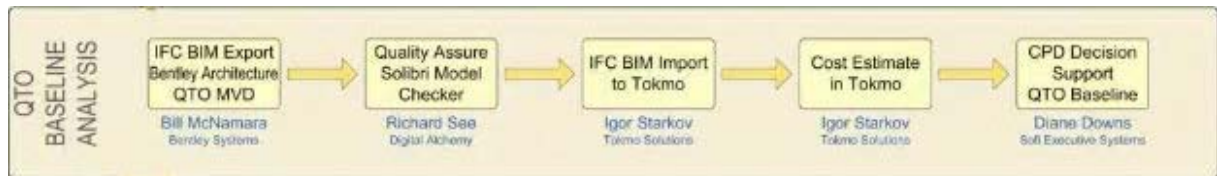
Figur 38. AECOO-1 QTO workflow diagram (OGC et al. 2009)
