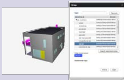
The Data Enricher allows users to attach IFD tags (panel, right) with detailed product information to the model, with further links (not shown) to the architectural model Source: Catenda
